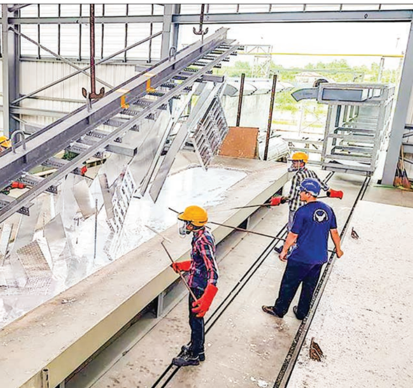
Hot-dip galvanization is a form of galvanization. It is the process of coating iron and steel with zinc, which alloys with the surface of the base metal when immersing the metal in a bath of molten zinc at a temperature of around 840 °F (449 °C). PHOTO: SCI METAL TECH MYANMAR CO., LTD.
