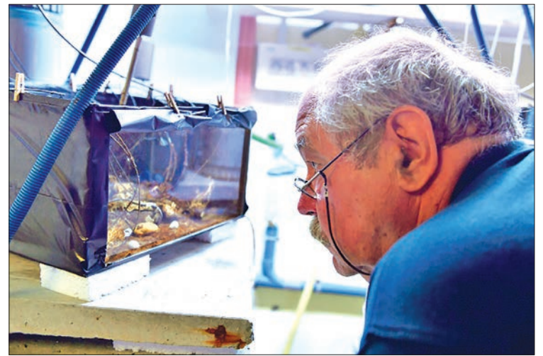
Jean-Charles Massabuau observing oysters attached to electrodes in a specially built tank at his lab in Arcachon, southwest France. PHOTO: AFP
