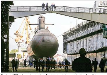
Project 677 submarines of the Lada class belong with the fourth generation of diesel-electric subs. **PHOTO: AFP**
